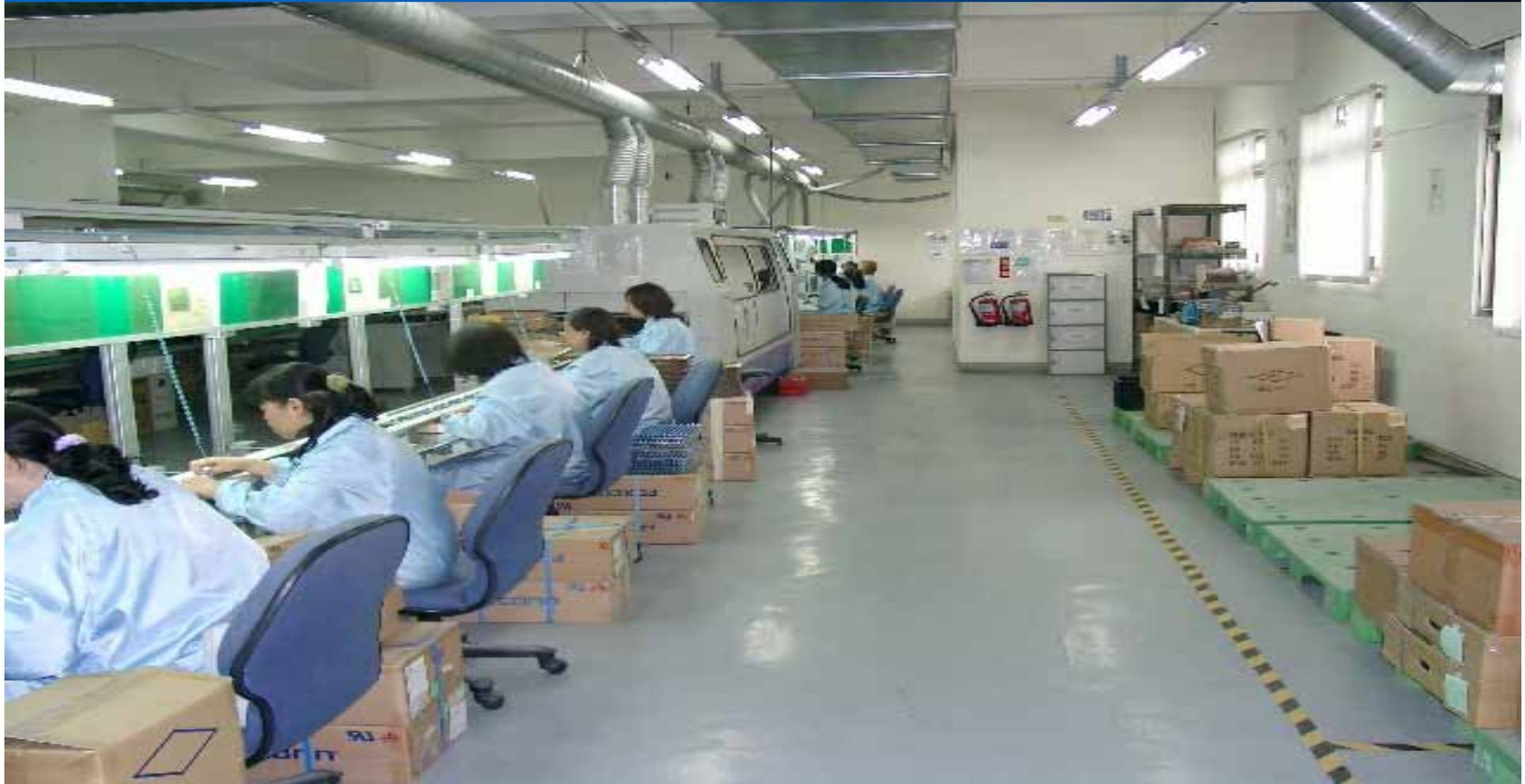
Insertion line (Double side 9M)+Wave solder (4M)
