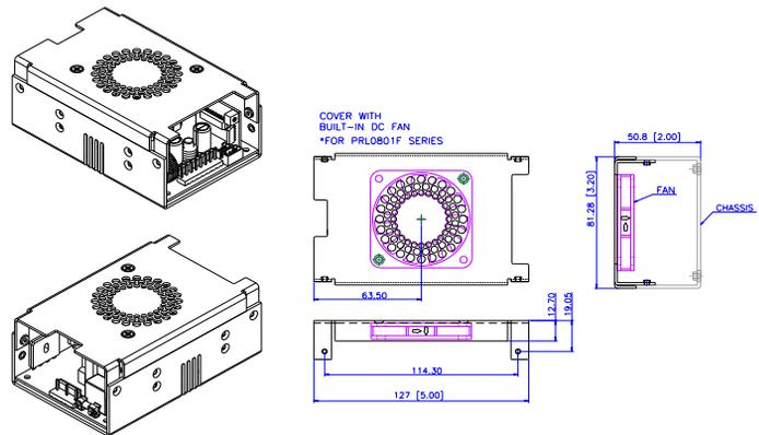
E Type (Enclosed with Rear Side built-in Fan): 6.5(L) x 3.2(W) x 1.6(H) inches; Weight: 650g.
