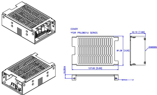
F Type (U-Chassis with Top built-in Fan):
